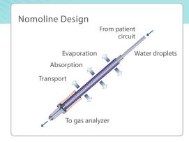
Nomoline fluid protection technology incorporates a unique sampling tube made of a special polymer water separation section - the *nomo* section and a bacterial filter. Unlike traditional solutions that remove water vapor or collect water in a plastic container, the Nomoline removes aspired or condensed water. Water passes through the membrane-like surface of the Nomoline and evaporates into the surrounding air, while leaving oxygen, and carbon dioxide gases unaffected.
